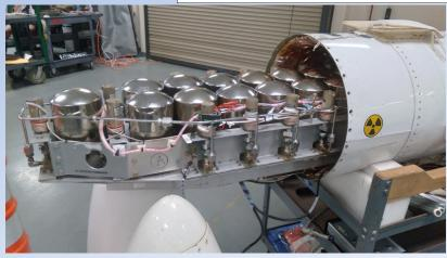
1. Manifold in ER-2 belly pod (nose cone off)
